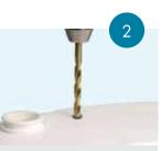
Drill a 10mm-diameter hole on top of the case where indicated.
